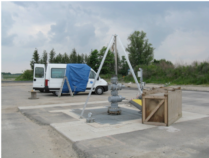
OGS transporter as mobile measurement cabin for the passive seismic recording via 3C-downhole receiver in observation well Ktzi202 (photo: courtesy of GFZ).
