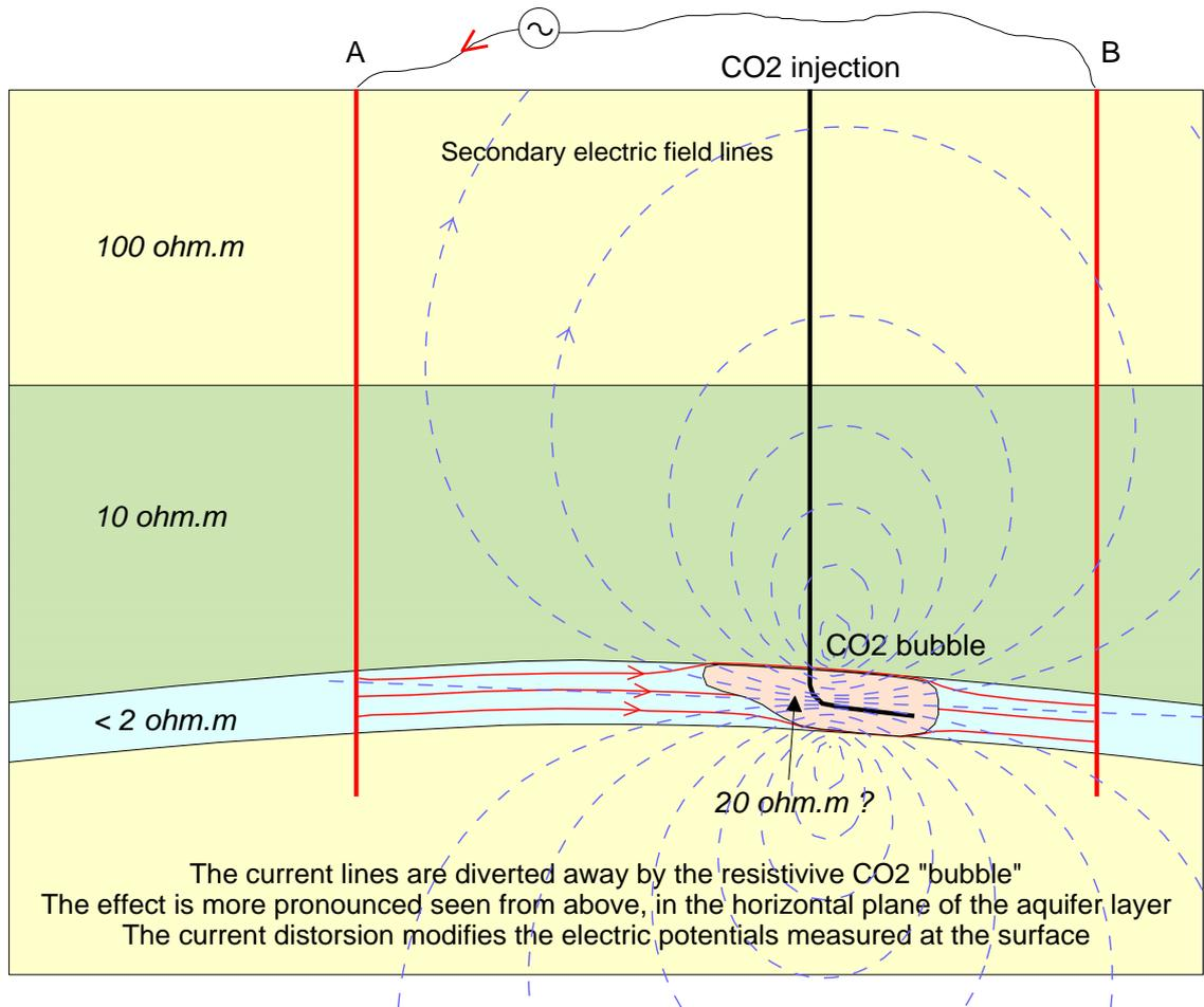
Figure 3 Concept of LEMAM electromagnetic monitoring techniques (BRGM)
