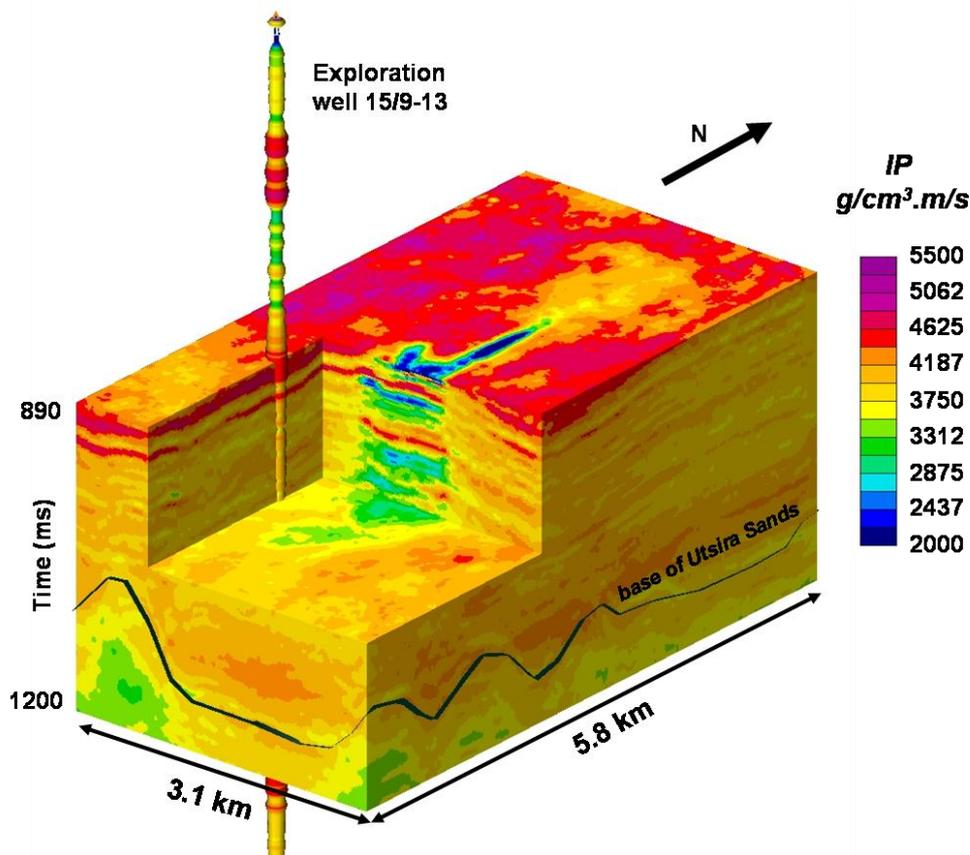
Figure 7 Cut-away view of the 3D P-wave impedance data cube computed by pre-stack stratigraphic inversion of the 2006 vintage. The figure also shows the exploration well used for the calibration step and the intersection between the base of the Utsira Sand formation with the boundaries of the cube. The CO<sub>2</sub> plume is identified by low impedance values displayed in dark blue, blue and green colours (IPEN).
