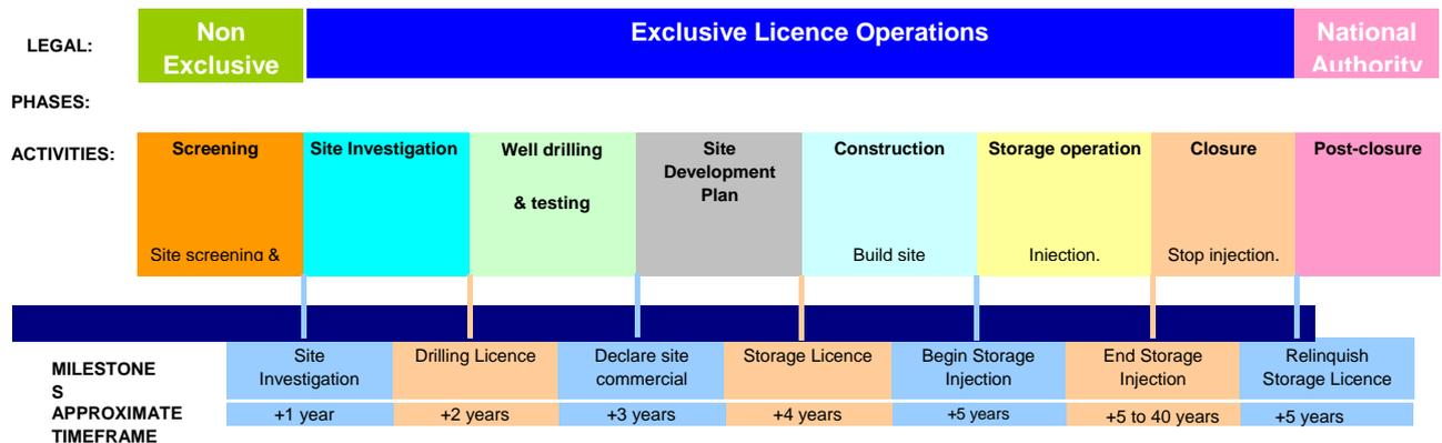
Figure 8 Phases in the realization of a CO<sub>2</sub> storage operation
